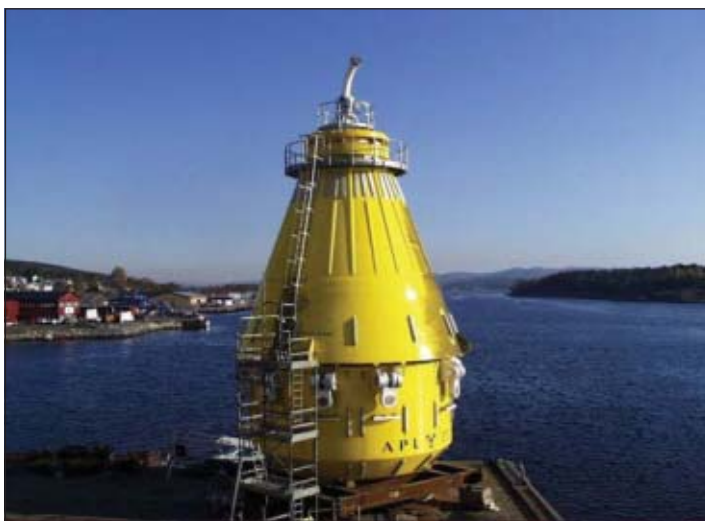
Advanced Productions and Loading AS's submerged buoy is one of the types of equipment used to unload natural gas from ships at offshore ports (photo from Advanced Production and Loading AS; Fig. 4).
