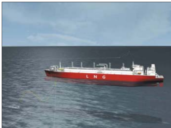
Excelerate Energy's Gulf Gateway Energy Bridge offshore port began LNG operations off Louisiana in 2005. Similar systems could be used both to load and unload CNG vessels (photo from Excelerate Energy; Fig. 2).
